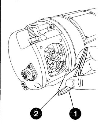
Detach cable connections (1) (plugs and jacks) of terminals 50, 50z, 48, 30 and terminal 30F to socket.
